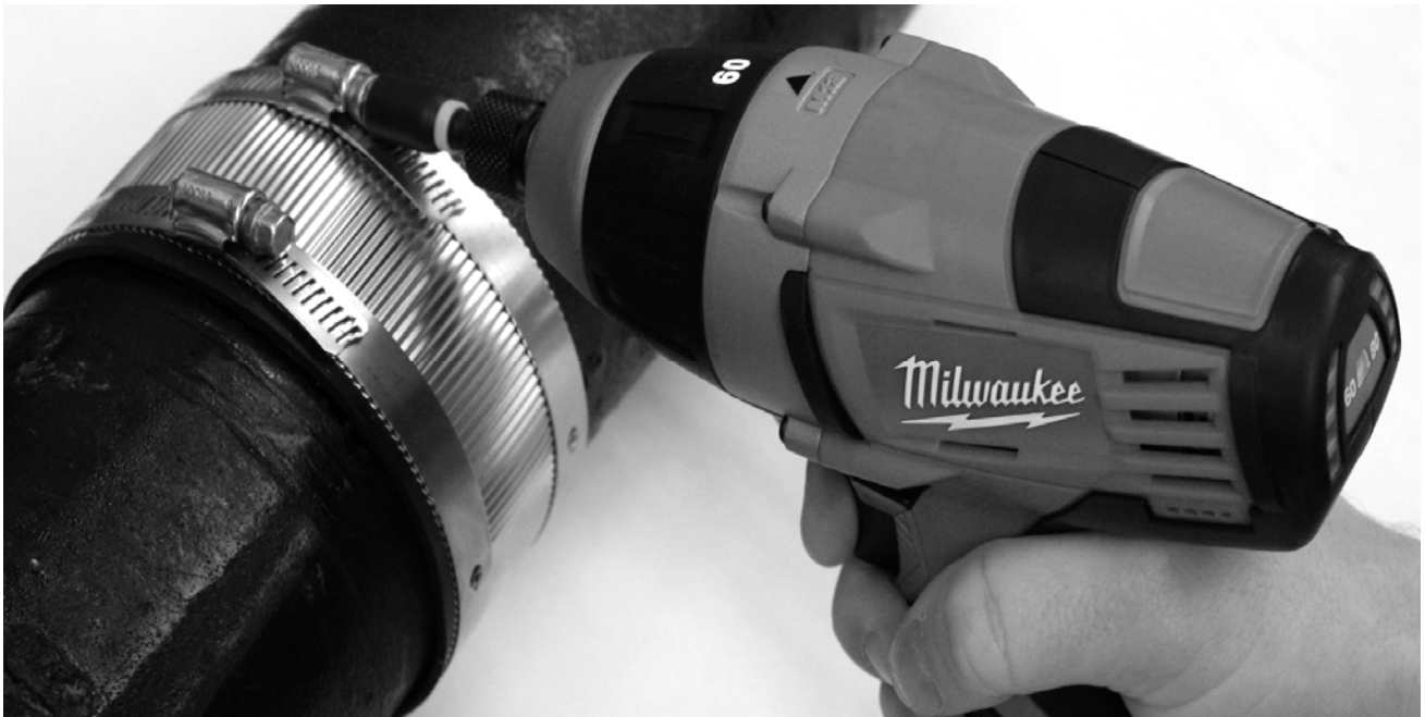
Typical power operated torque tools used for coupling assembly.
